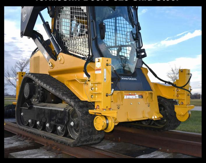
Model 6060 Flexiride Rail Gear for Skid Steer Loaders has 4-wheel independent hydraulic suspension. The hydraulic system is independent of the machine hydraulics. The rail gear mounting kit is welded to the machine frame and the rail gear assemblies bolt to the mounting kit.
